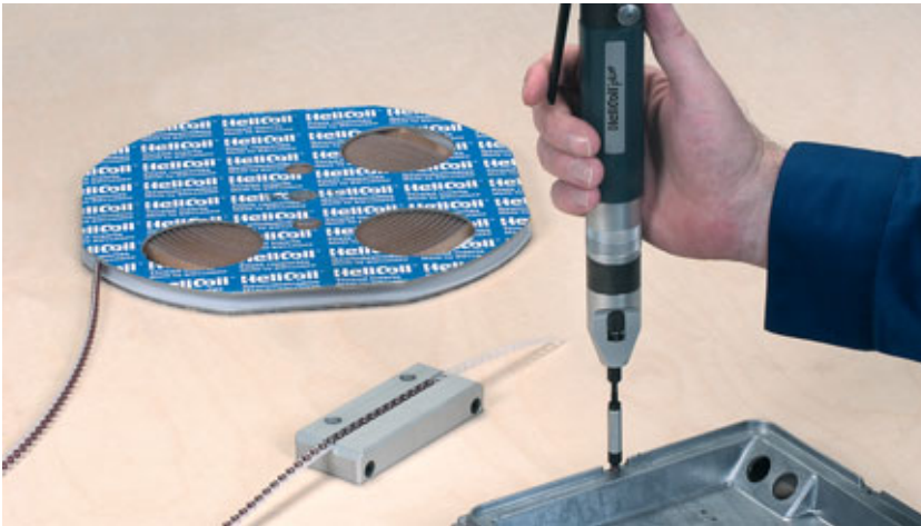
Installation of HELICOIL® plus
